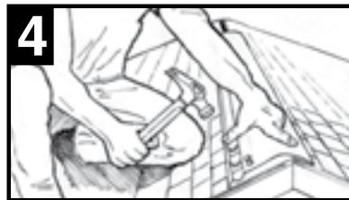
Apply the vent so that the hinge is centered along the peak allowing the flange to rest on the roof deck (**see view 4a**) opposite the slot opening. Secure roof vent body using 2.5" ring shank roofing nails and nailing through (2) provided pilot holes on vent body.
